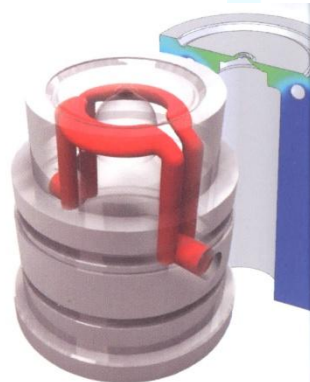
conformal cooling 11 seconds
